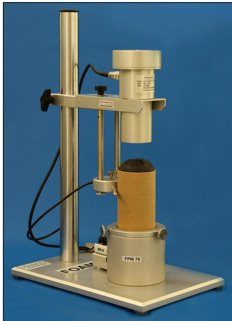
**Fig. 1:** The new Foam Pressure Measurement Device FPM 70 on the stand of the Foam Qualification System FOAMAT®. Rise height, rise pressure and reaction temperature are measured simultaneously.
