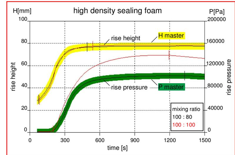
**Fig. 3:** Two rise height and rise pressure profiles of a high density sealing foam. The mixing ratio was changed from 100:80 to 100:100. The master curves can be adapted to acceptable QC margins.
