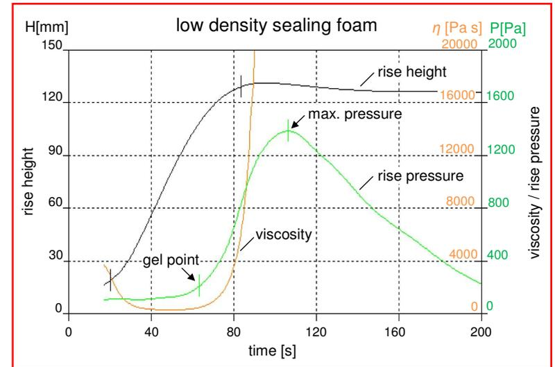
**Fig. 2:** Rise height, rise pressure and viscosity of a low density sealing foam measured with the FPM 70. The viscosity data is calculated by using the physical model of Hagen-Poiseuille.
