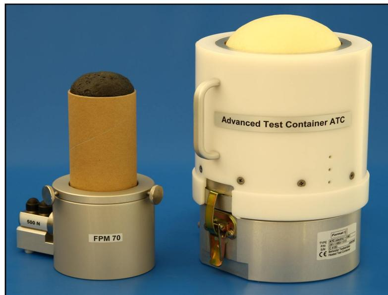
**Fig. 4:** The new Foam Pressure Measurement Device FPM 70 compared to the Advanced Test Container ATC. The test volume is reduced down to 15%.
