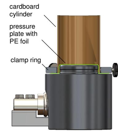
**Fig. 5:** Cross section of the new FPM 70, designed for the pressure measurement of high density foams.
