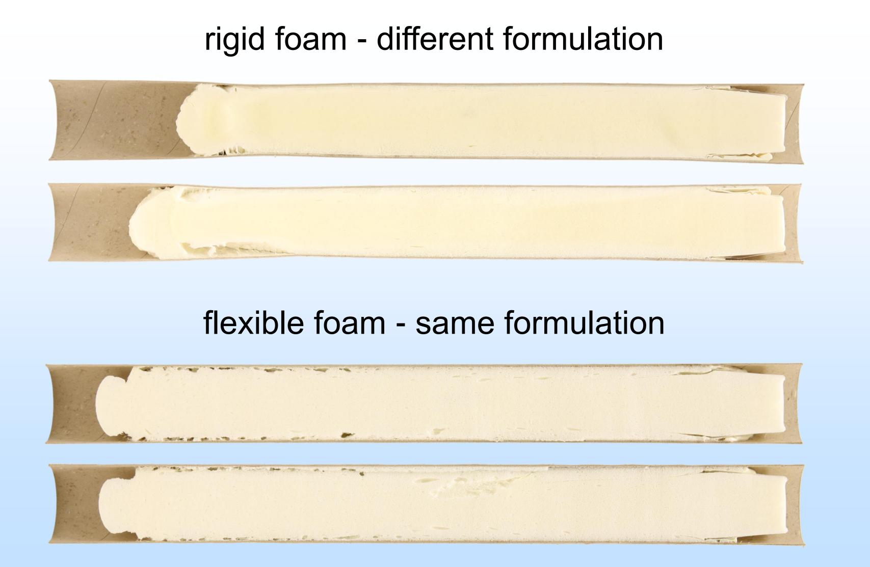
Fig. 4: Lance Test procedure. After mixing, the cup is dropped into the cardboard cylinder to slide down onto the pressure sensor. The expanding foam is measured contactless by the ultrasonic sensor LR 4 and the rise pressure by the FPM 2.
